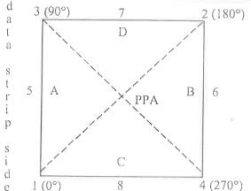
Positions of all points are referenced to the principal point of autocollimation (PPA) as origin. The diagram indicates the orientation of the reference points when the camera is viewed from the back, or a contact positive with the emulsion up. The data strip is to the left.
